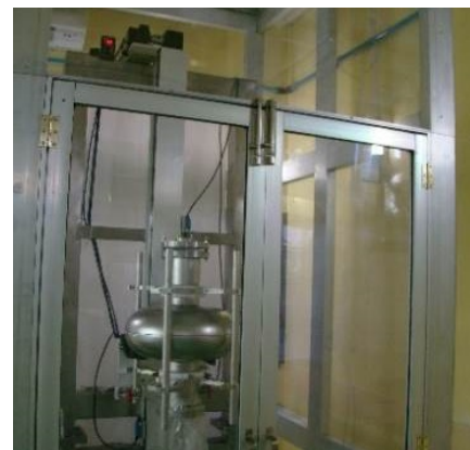
High pressure rinsing (@ 100 bars pressure)
