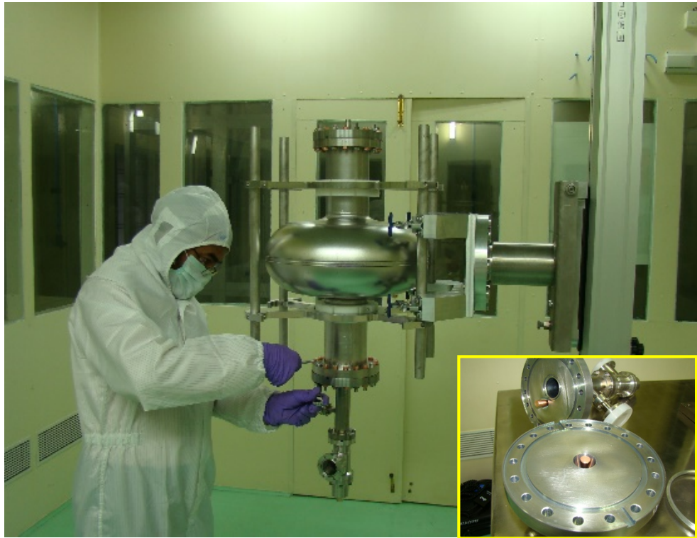
Cleanroom assembly of 650 MHz cavity at RRCAT
