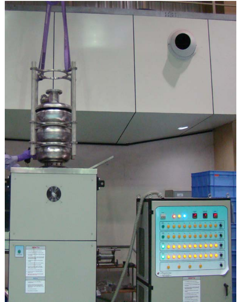
Ultrasonic cleaner for five-cell 650 MHz cavity at RRCAT
