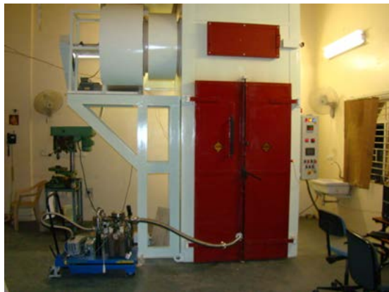
Low temperature baking (@ 120°C for 48 hours)
