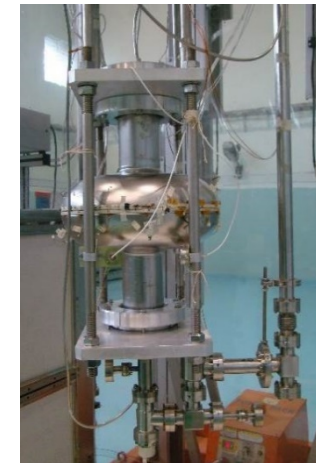
Cavity loaded on VTS insert assembly for 2 K testing)
