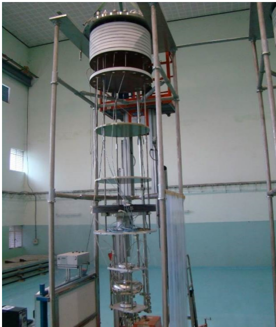
Single-cell 650 MHz cavity in VTS Cryostat
