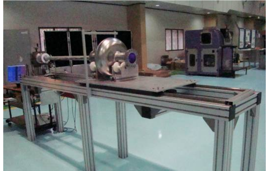
Inspection of single-cell 650 MHz cavity
