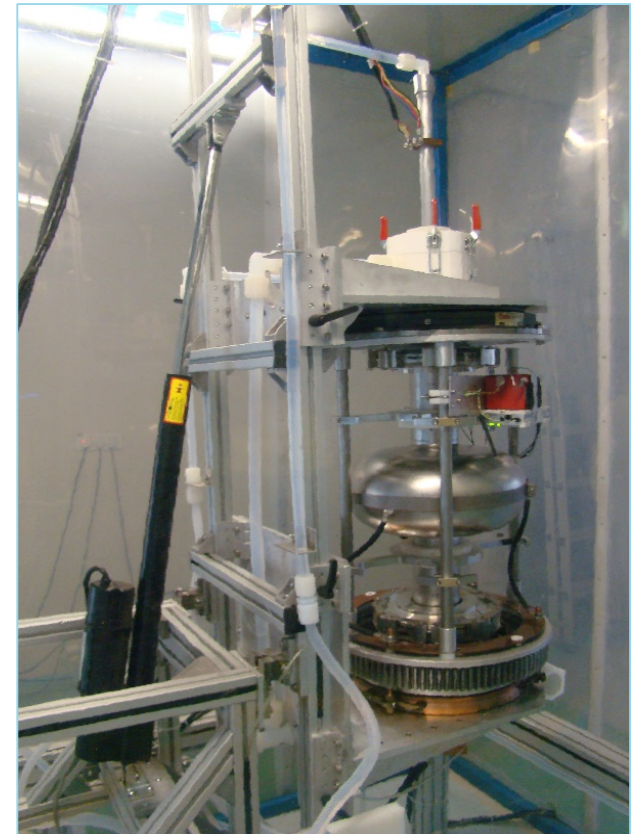
Cavity moved to vertical position for draining of electrolyte, rinsing of cavity and For insertion/removal of cathode
