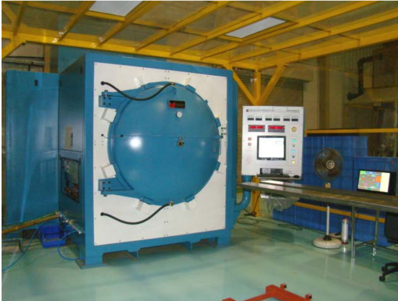
High Vacuum Annealing Furnace at RRCAT
