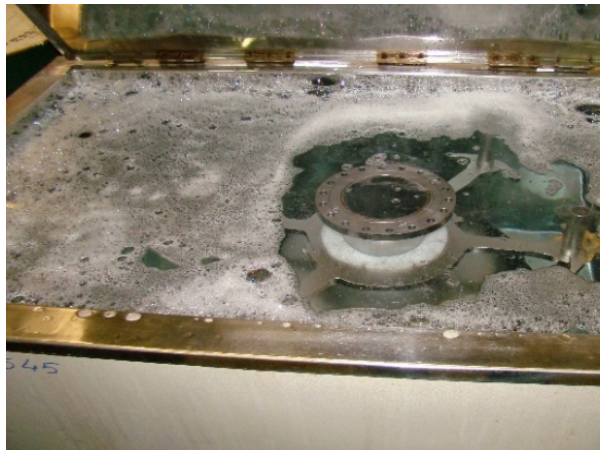
Ultrasonic cleaner for small components & single-cell cavities at RRCAT
