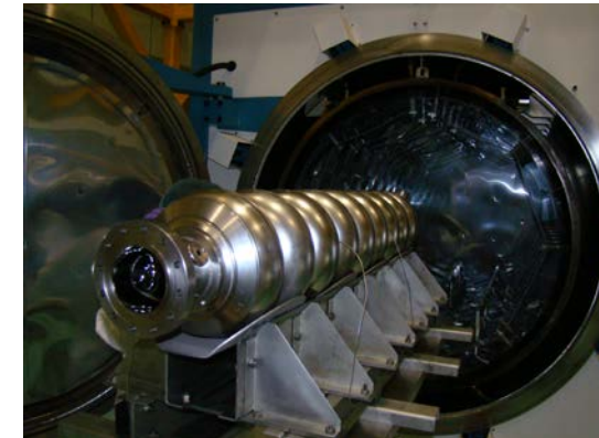
Nine-cell 1.3 GHz cavity prepared for annealing
