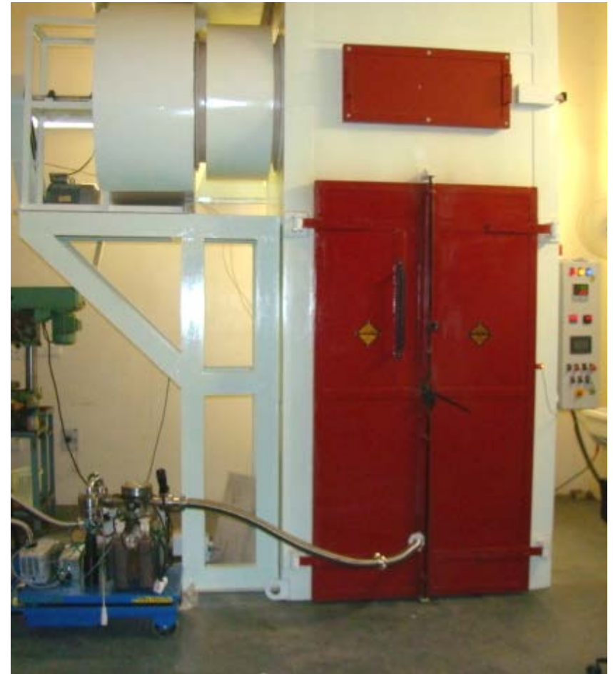
120 C Hot Air Baking Facility at RRCAT
