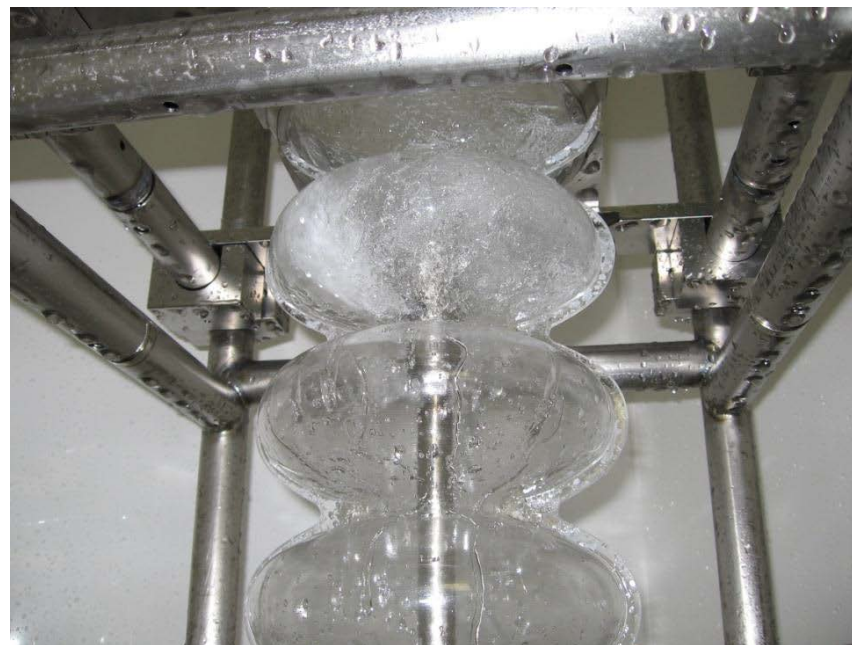
High pressure water jets during HPR
